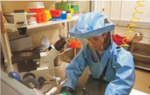
A researcher working with the Ebola virus while wearing a BSL-4 positive pressure suit to avoid infection
